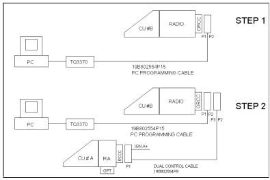
Figure 31 - ORION Dual Control Unit PC Programming Configuration
